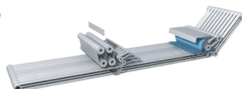
3rd Cross Fold – Reversing conveyor and blade.
