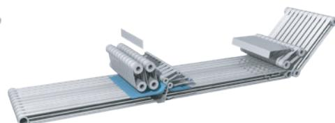
2nd Cross Fold – With blade. New system to support linen throughout the folding phase and avoid problems with slippages.
