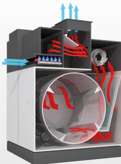
air flow with recirculation for ST2700/G
