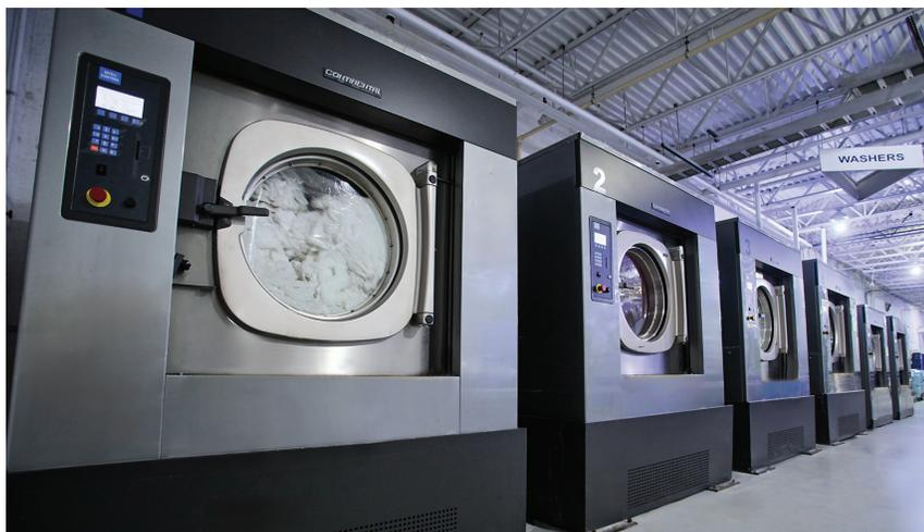
**Open-Pocket Washers:** Continental and Girbau Industrial (GI) open-pocket soft-mount washers (20- to 255-pound capacities) are highly efficient with extract speeds reaching 450 G-force. The high extract removes more moisture from every load, which cuts drying time by up to 50 percent. This means dryers complete loads in half the time, using half the natural gas. The shortened wash/dry time maximizes throughput and allows operators to complete more loads in less time — saving labor.
