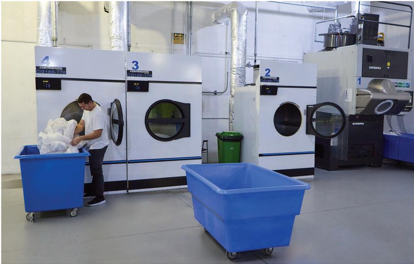
**Dryers:** Continental and GI Dryers are highly flexible and designed to contain heat and optimize air flow for unrivaled efficiency. Some models offer suction loading and the ability to work in concert with a tunnel washing system or as a stand-alone unit.
