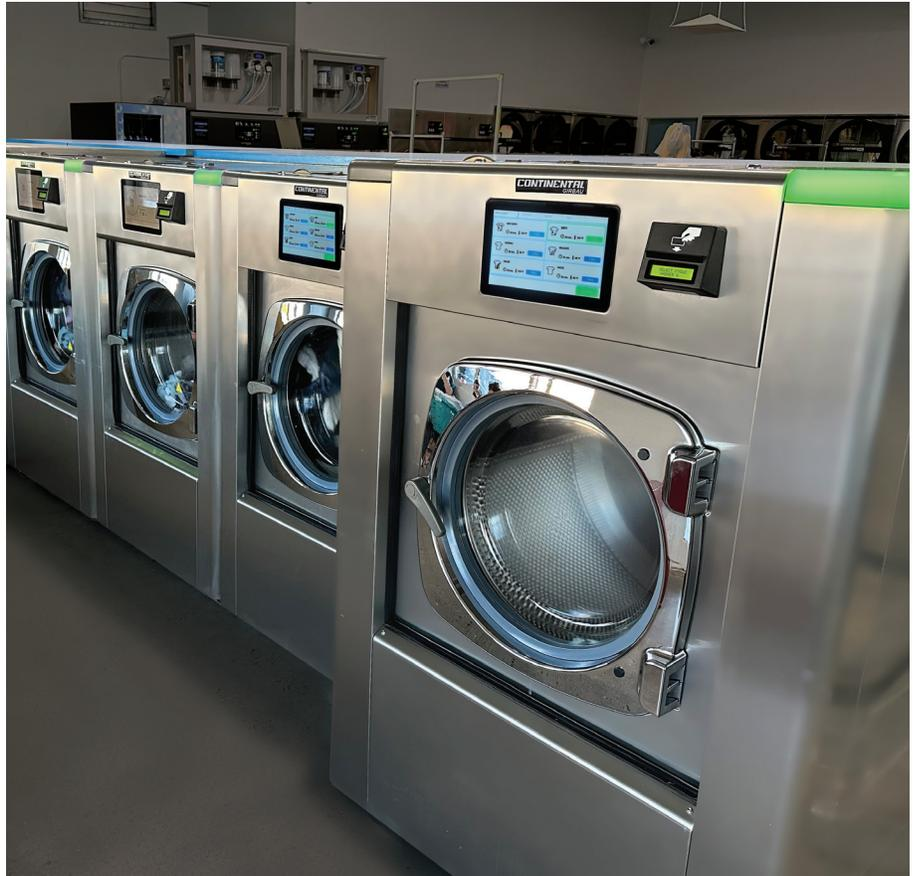
The new soft-mount washers, which replaced aged-out, lower speed hardmounts, generate up to 450 G-force extract for more moisture removal and reduced dry times. In doing so, they've also cut natural gas costs and improved customer rotation rates, according to Quispe. Now, customers are in and out in 60 minutes or less ...
