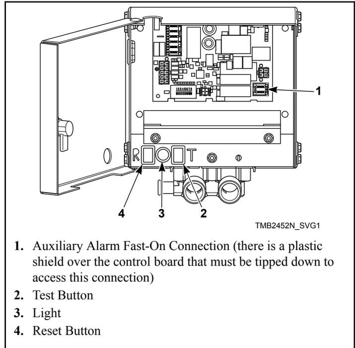
1. Auxiliary Alarm Fast-On Connection (there is a plastic shield over the control board that must be tipped down to access this connection)
