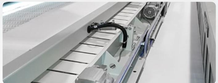
A highly recommended option for improving feeding quality even further. A number of smoothing belts located above the discharge conveyor, along with a series of brushes on 1 or 2 lanes, depending on the feeder chosen, correct any imperfections which may have appeared.
