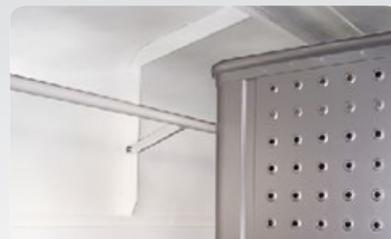
The steel rail prevents the laundry transporting carts from hitting the feeder and helps the operators to access the carts and their loads.
